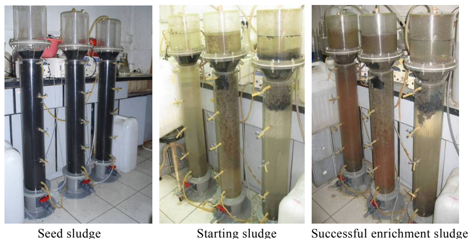
图 1 反应器启动过程污泥颜色变化情况 (从左到右依次是空白、多面空心球和竹炭反应器) Fig. 1 Changes in appearance UASB reactor during the whole start-up experiment (from left to right CK, SP and BC reactor, respectively).
